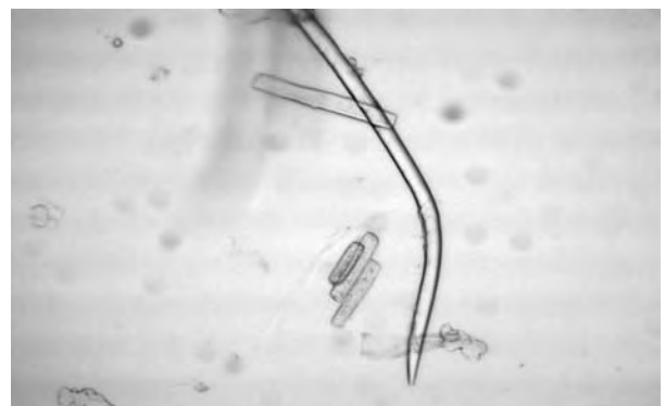
Fig. 37 Fibre di Themeda arundinacea Roxb. con forma cilindrica e terminazione a punta d'ago (100x). Themeda arundinacea Roxb. fibers as a cylindrical shape and end-point termination (100x).
